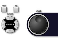
You select parameters and objects with a left click. You change the selected parameter's value by turning the scroll wheel. You can display an object's menu by right-clicking the object.
